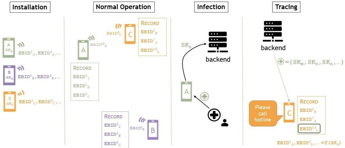
Figure 1: Phases in the decentralized proximity tracing system
